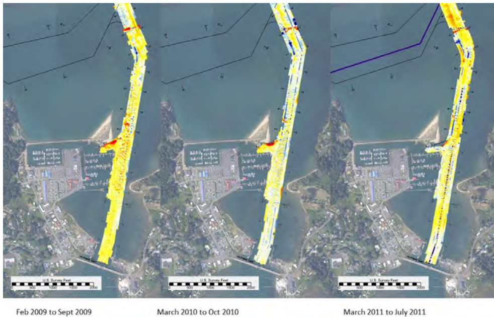
Figure 3. Example analysis- Charleston Marina, Coos Bay, depth differences between sequential pre-dredge and preceding post-dredge surveys
